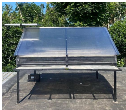
Gambar 3. Alat solar dryer portable berbasis IoT
