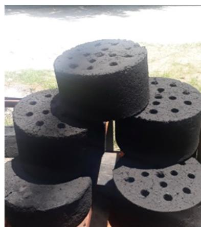
Gambar 6. Briket Ampas Sagu 14 Lubang
